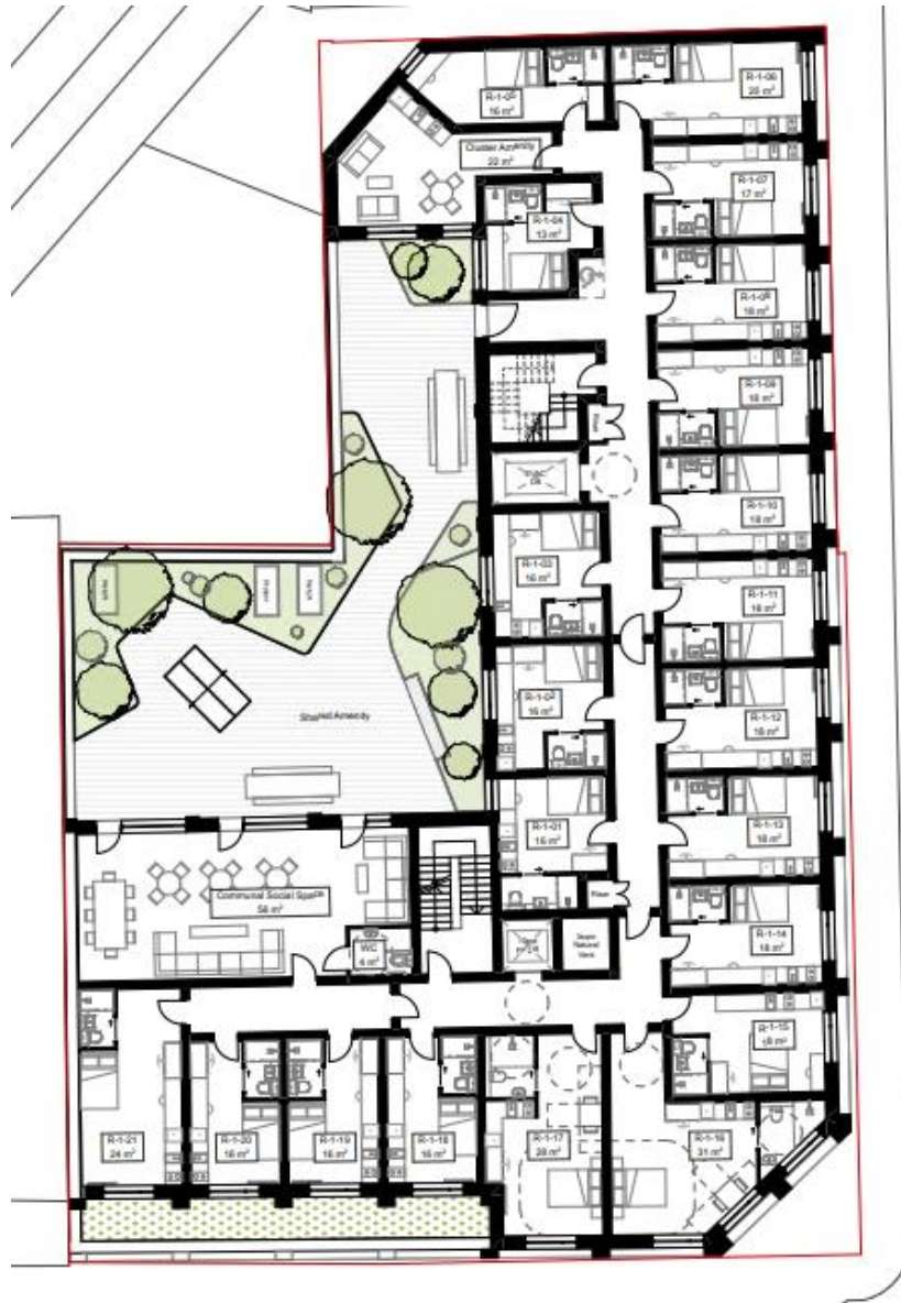
Proposed First Floor Layout – comprises communal social space, outdoor amenity space and student units (2 x cluster units located to the northern part and studio units within the central and southern part).
