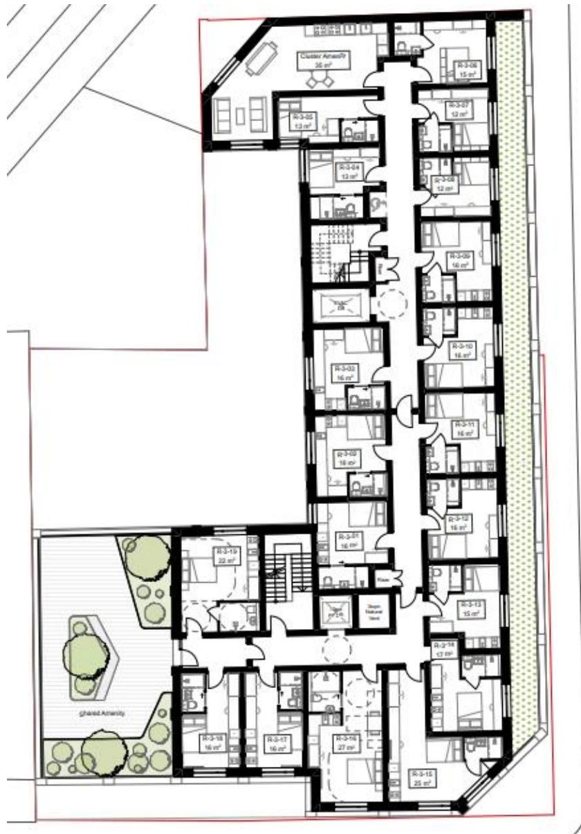
Proposed Third Floor Layout – this plan demonstrates 5 x cluster units located at the northern part of the site and 14 x studio units on the central and southern part of this floor. There is a third floor terrace located on the western side of the site.
